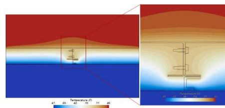
Vertical temperature distribution on the AHU panel
