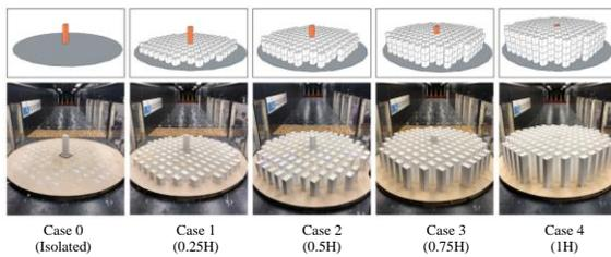
Different test configurations used in the experiments
