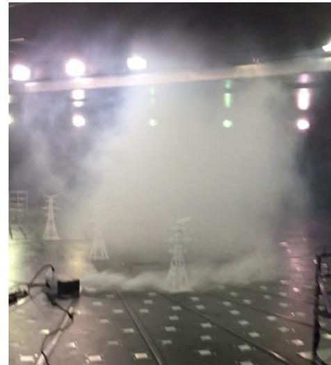
Aeroelastic multi-span transmission line model under a simulated tornado conducted in WindEEE research institute
