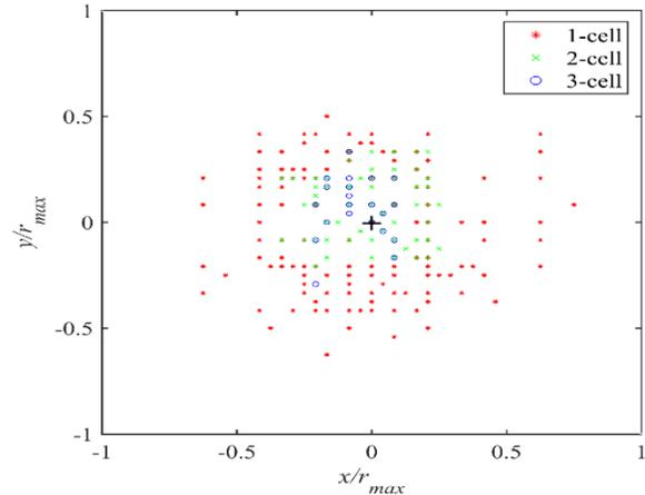
Fig. 1. Distribution of vortex centers in the 1-, 2-, and 3-cell structures of Mode B TLVs around the center of the turntable (the elapsed time from 0 to 30 s with a frequency of 20 Hz for  $S=0.853$  and normalized by  $r_{max}=1.2$  m).
