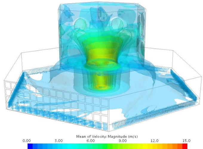
CFD Simulation of a tornado-like vortex in the WindEEE Dome
