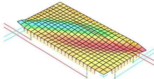
Out of plane deformation of sheathing panel due to pure shear – Finite Element Model
