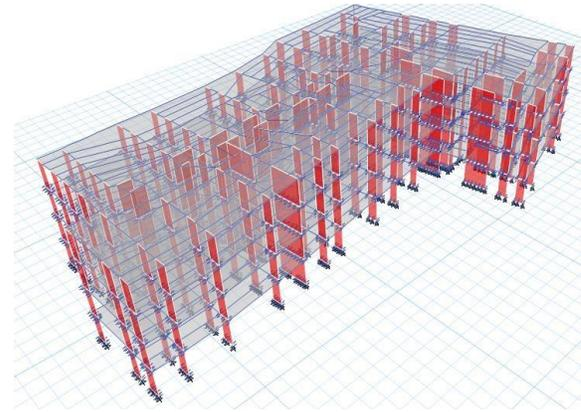
Numerical model showing the formulation of CLT panels as shear walls
