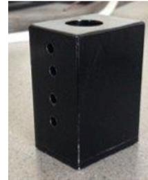
Figure 5 Model porous geometry with a gradually decreasing hole size down the centre, and viewing holes in the side through which thermocouples are inserted
