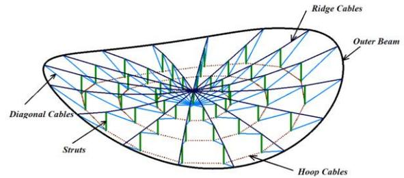
Components of a negative-Gaussian curvature cable dome
