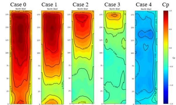
Mean pressure coefficients (Mean Cp's) on the Northern wall for 0° angle of attack
