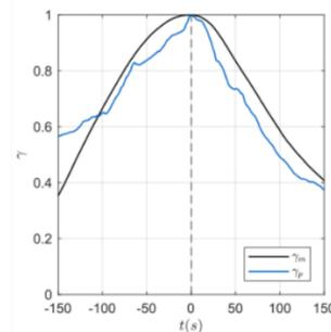
The  $\gamma$  function of the full-scale downburst event ( $\gamma_p$ ) and the WindEEE Dome reconstruction ( $\gamma_m$ ).
