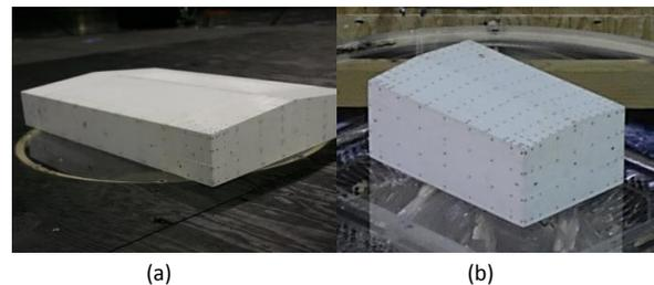
Figure 1. Building models (a) Large building, and (b) Small building
