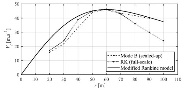
Fig. 2. Comparison of radial profile of the tangential velocity in scaled-up Mode B TLV (1:6.5 for velocity and 1:50 for length) and RK tornado. Vertical profiles are matched at  $r_{max}=60$  m.
