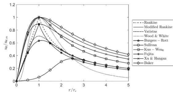
Radial profiles of tangential velocity calculated using different analytical models of tornadoes. Apart from Rankine and modified Rankine vortex models, the shape of all other profiles can be manipulated depending on the choice of model parameters.
