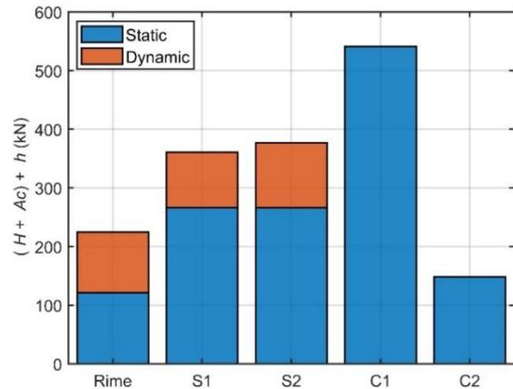
Fig 2. Static and dynamic effects transmitted to the tower due to wind and ice loading
