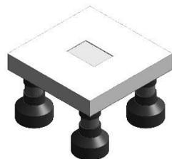
The experiments examined the movement of a 1:150 geometrically scaled platform with six degrees of freedom and two mooring Configurations. Four Configurations are studied, (1) Loosely moored platform, (2) Tightly moored platform, (3) Platform with ballast, and (4) Platform with ballast and weight on the deck.
