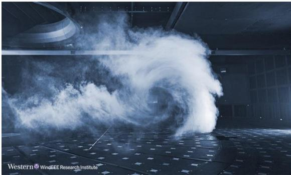
WindEEE's different flow configurations can be used to determine pressures and dynamic response of various structures. Scale models of buildings (residential, commercial, industrial, hospital, high-rise), bridges, transmission towers, wind turbines and many others can be tested. Various techniques are used to simulate the effect of surrounding buildings, topography and canopy in order to replicate the local site conditions.
