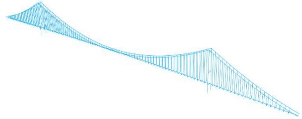
Finite element model of a suspension bridge
