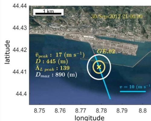
Reconstructed location of a full-scale downburst close to Genoa (Italy) using WindEEE Dome simulations
