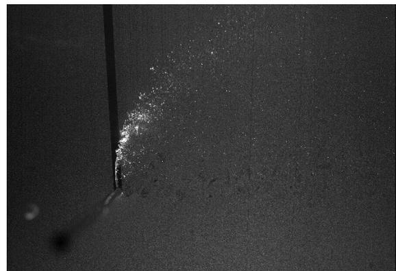
Figure 8 - Particle image velocimetry image of the JIC (crossflow direction: left-to-right)
