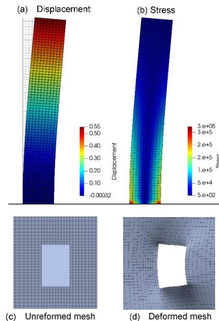
Result of fluid-structure interaction for CAARC model under wind load: structural response (a), stress (b), unreformed mesh(c) and deformed mesh (d)
