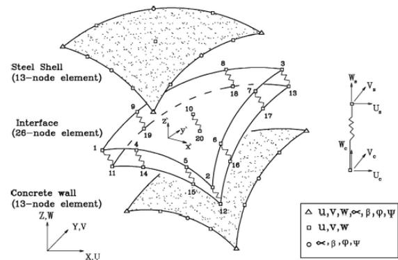
Elements used to model steel and concrete walls in addition to interface between concrete and embossed steel plate (after Elansary and El Damatty 2017)
