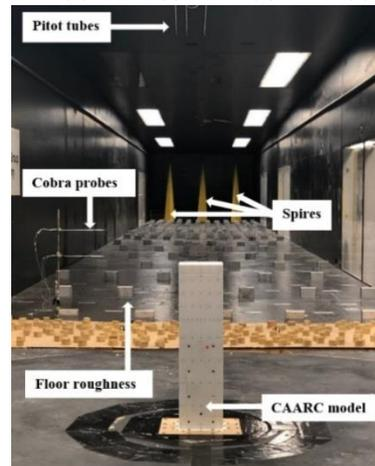
Experimental model installed at (UWO WIND TUNNEL) for the Isolated case 0 at AoA=0°
