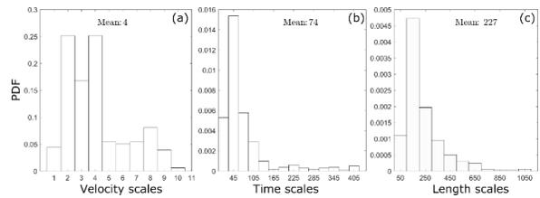
The WindEEE Dome downburst scales: (a) velocity (mean flow), (b) time and (c) length scales.
