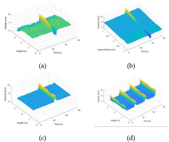
3D pictures of the time history of the turbulent velocity field, (a) EVS, (b) EHS, (c) EOG generated with changing fan powers, (d) EOG generated with IGVs
