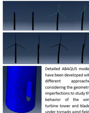
Detailed ABAQUS models have been developed with different approaches considering the geometric imperfections to study the behavior of the wind turbine tower and blades under tornado wind fields
