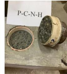
Experimental shear lap and pull-off tests used to study the shear and peel behavior of concrete – embossed steel plates
