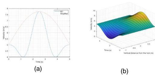
The scaled extreme conditions for simulations and experiments based on the micro wind turbine and capability of the fans, (a) extreme operating gust, (b) extreme vertical shear
