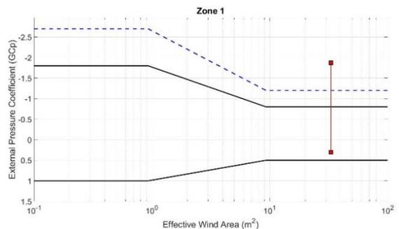
Fig. 3. Maximum and minimum enveloped pressure coefficient in zone 1 compared to ASCE 7 provisions.
