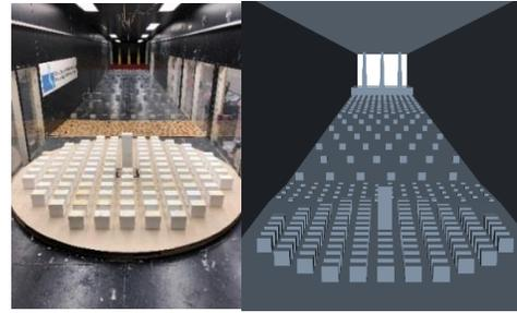
Wind Tunnel Testing and CFD Simulation
