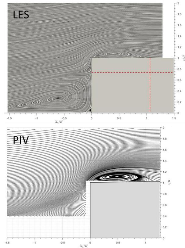
Fig. 2: Mean velocity streamlines comparison between LES and PIV measurements over a vertical section cutting through the centerline of the building in the flow-direction
