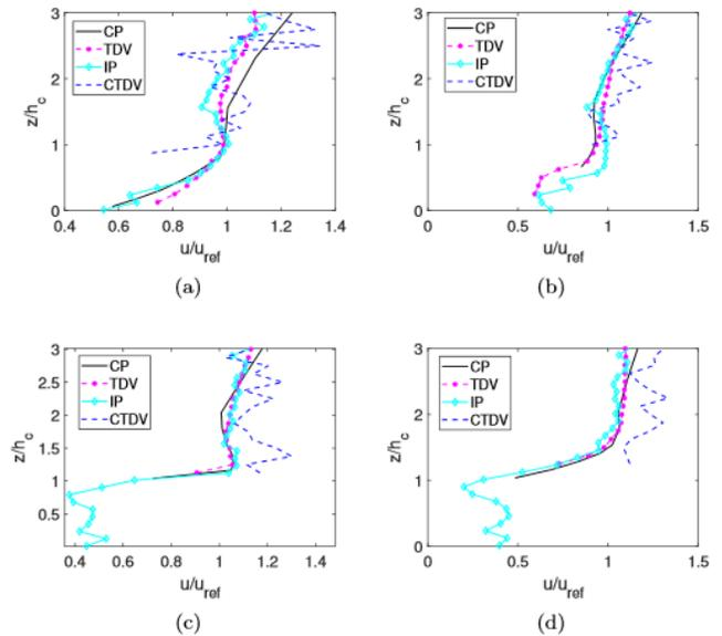
Impact probe (IP) and Cobra probe data (CP) versus TDV and CTDV results - normalized  $u$  component in (a)  $x = -1.5hc$ ; (b)  $x = 0$ ; (c)  $x = 1.5hc$  and (d)  $x = 3.375hc$ . The variable  $hc$  is the forest canopy height which is 400 mm
