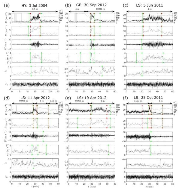
Change points detected using the M (red line) and SD (green line) methods applied to decomposed velocity records (subplots) of the several (a–f) thunderstorms from Europe.
