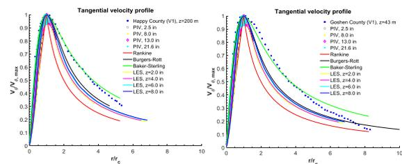
Particle Image Velocimetry (PIV) measurements of tornado-like vortices from WindEEE Dome for swirl ratios deemed representative of the Happy county (V1) and Goshen county (V1) tornadoes based on the scaling technique developed by Refan et al [2] are used for comparing the experimentally generated flow-field. High fidelity Large Eddy Simulations (LES) of tornado-like vortices are also conducted using a simplified cylindrical computational domain with uniform, steady input velocity.
