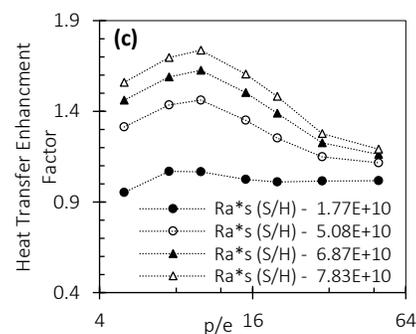
Fig 1c. The effect of roughness spacing
