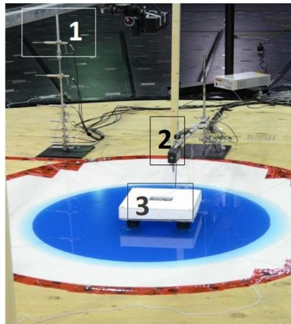
Instrumentation Set-up: (1) Cobra Probes, (2) Resistance wire wave probe (3) Floating platform with the IMU and accelerometers. The ABL wind is coming from left.
