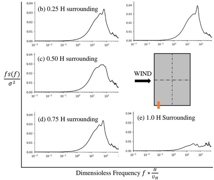
Power spectral densities of pressure at model height of 0.96H for (a) Cases 0, (b) Case 1, (c) Case 2, (d) Case 3, (e) Case 4 in Suburban
