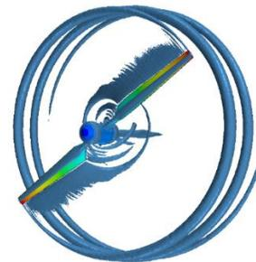
Vorticity surface of operation NASA Phase VI turbine under 5 m/s mean wind speeds
