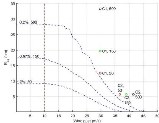
Fig.1. Hazard contours representing three different reliability levels and the radial ice accretion speed data pair for a 10 m/s wind speed
