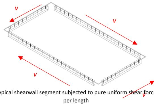
Typical shearwall segment subjected to pure uniform shear force per length
