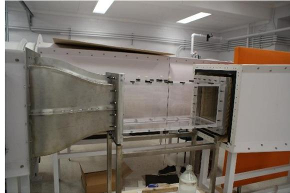
Figure 7 - Wind tunnel contraction and test section containing a 4mm spray bar
