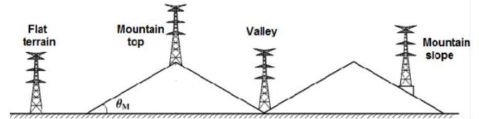
Transmission line on different terrains and topography
