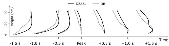
Evolution of DB and DBABL radial velocity profiles at a fixed position in the outflow. Velocities are normalized with the maximum velocity, while the height (in cm) and time (in s) are not normalized.
