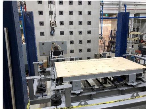
Shear buckling test set up
