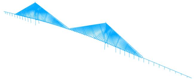
Finite element model of a cable-stayed bridge
