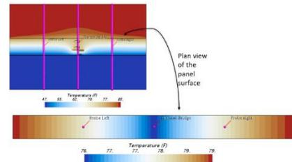
Horizontal temperature distribution on the AHU panel
