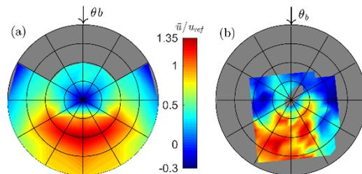
Normalized radial velocities in the DBABL outflow in the WindEEE Dome (a) and real downburst observed using Doppler radars (b). The incoming direction of background ABL winds denoted with  $\theta_b$ .
