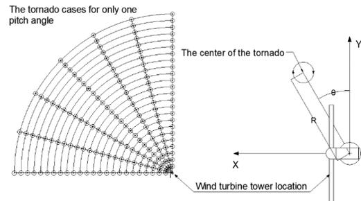
Schematic of tornado locations for the current study relative to the centerline of the wind turbine
