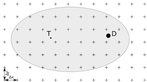
A 3-km grid is represented with black crosses. The symbols T and D represent a 300-m and a 1000-m wide tornado and downburst, respectively. The shaded ellipse is an idealized contour of a thunderstorm cloud. In this case, both tornado and downburst are sub-grid processes that cannot be directly resolved on this coarse grid.
