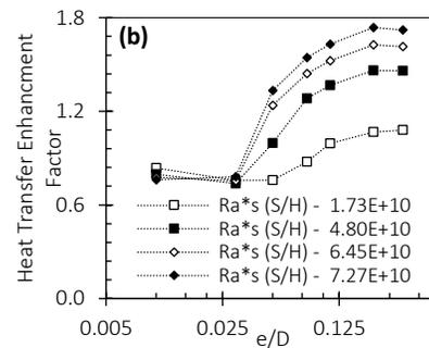
Fig 1b. The effect of roughness height
