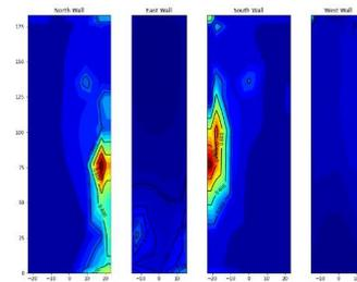
Overall Fatigue Damage at 1/4 H Surrounded Case
