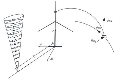
Velocity components of the tornado wind field for a random element in the coordinate system
