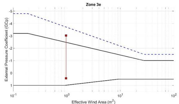
Fig. 4. Maximum and minimum enveloped pressure coefficient in zone 3e compared to ASCE 7 provisions.
