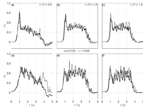
Time histories of drag coefficient ( $c_D$ ) on C125 (black) and C040 (grey) cylinders immersed in the DB and DBABL outflows (two rows) at three different  $r/D$ s (three columns). The values are provided at  $z/L = 0.056$  (i.e., 5 cm) above the ground.
