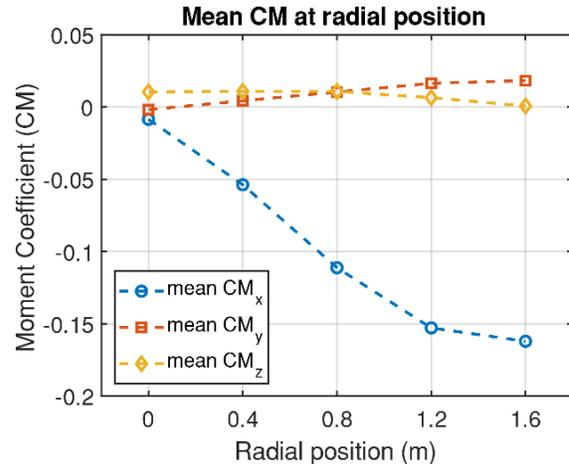
Mean CM at different radial locations with respect to the tornado vortex center for the parked rotor mode.  $CM_x$  is the bending moment and  $CM_z$  is the twisting moment of the wind turbine.
