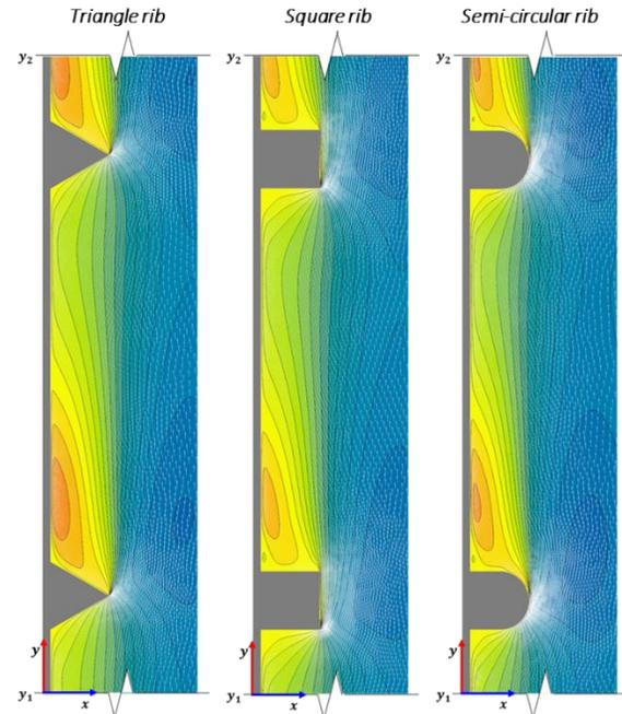
Fig 1a. Typical flow structures between consecutive ribs
