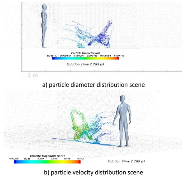
Figure 1. Preliminary unsteady cough jet propagation model
